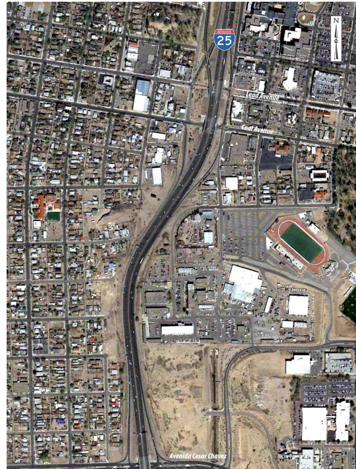
Exhibit 1-2, Key Deficiency in the South I-25 Corridor – 50 MPH S-Curve
